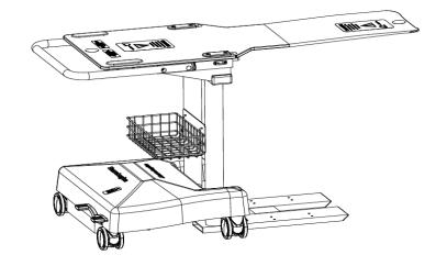
0-00202-001 Option, Extended Scanboard Long Post With Target A356.0 Aluminum, 304 Scanning platform
